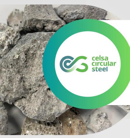
LFS - LADLE FURNACE SLAG B - (GRANULATED)
