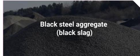
This is derived from the processing of black slag generated during the process of manufacturing steel in the electric arc furnace. It is used mainly as a raw material for the manufacture of surfacing, base and bed layers for roads.
