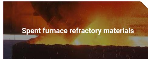
The main refractory materials used in the steel manufacturing process are masses of magnesium oxide (MgO), dolomite bricks and high-alumina bricks. Once they have worn out, most of these materials are reused in the steelmaking process itself, or as recycled raw materials to manufacture new refractory materials.
