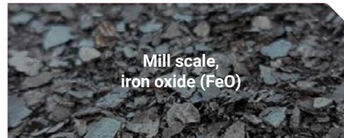
Produced mainly in the hot rolling process. This material is derived from the surface oxidation of the hot steel, and essentially comprises iron oxides. Its chemical composition allows it to be used in other industrial processes requiring an input of iron, such as primary steel manufacturing, cement and ferrous alloys.
